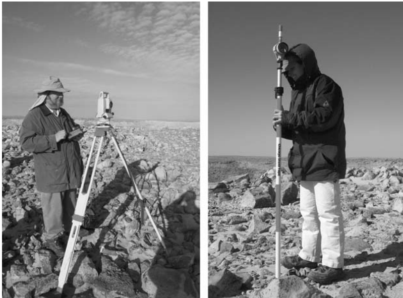
FIGURE 2.12 The use of total stations has revolutionized archaeological recording for both accuracy and speed. On the left, a crew member uses a small computer to coordinate information received from the total station. On the right, another crew member holds the prism pole at the point being recorded by the total station.
